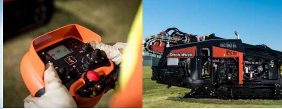
With the new **JT60 Horizontal Directional Drill**, you'll recognize many of the features you've grown to appreciate: the proven, intuitive electronics and the rugged, reliable undercarriage, to name two. And in no time you'll appreciate the JT60's more powerful rotational torque—an 80 percent increase over its predecessor the JT4020—and 60,000 lb (267 kN) of thrust and pullback. It's the powerful combination you needed—the combination you asked for—to work more efficiently with less downtime.
