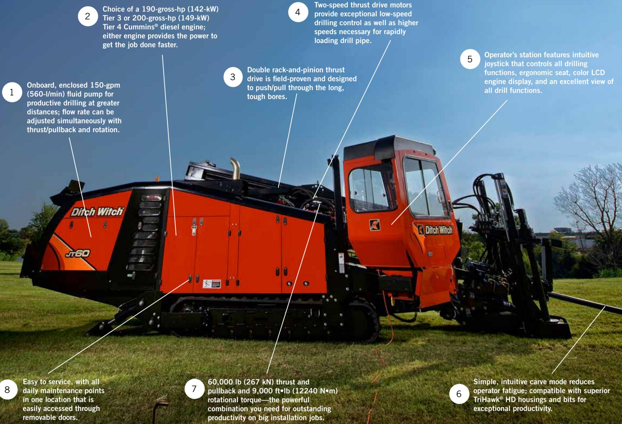
1 Onboard, enclosed 150-gpm (560-l/min) fluid pump for productive drilling at greater distances; flow rate can be adjusted simultaneously with thrust/pullback and rotation.
