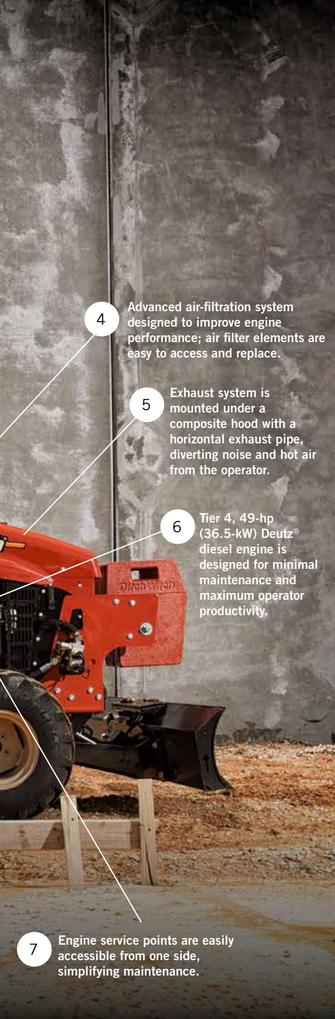
4 Advanced air-filtration system designed to improve engine performance; air filter elements are easy to access and replace.
