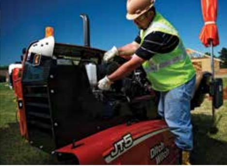
Experience built the **Ditch Witch®** **JT5 Horizontal Directional Drill**. With input from our customers and their many years of experience installing utilities on tight jobsites, our engineers developed the ideal compact rig with the right amount of thrust and pullback for shallow installations of cable, fiber and water systems up to 150 feet in length (46 m) beneath roads, driveways, sidewalks, sensitive landscaping, and other surface obstacles. The JT5 is a true team effort.
